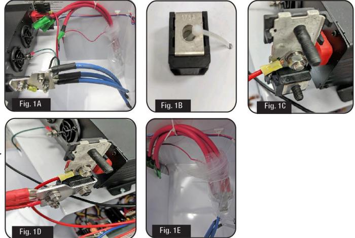
**CAUTION!** Do not install the battery fuse before making batteries wire connections. Failure to follow this recommendation can burn the battery wire connector or the battery terminal due to the electrical arc caused by the charge of inverter input capacitor.
